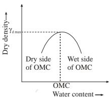
At dry side of OMC; dry density increases by increasing water content and at wet side of OMC, dry density decreases by increasing water content.
